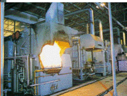
Hermetically sealed rectangle stove in the motorcycle components manufacturing plant in Qianjiang, China. Relau pemampat di kilang membuat komponen motorsikal di Qianjiang, China.
